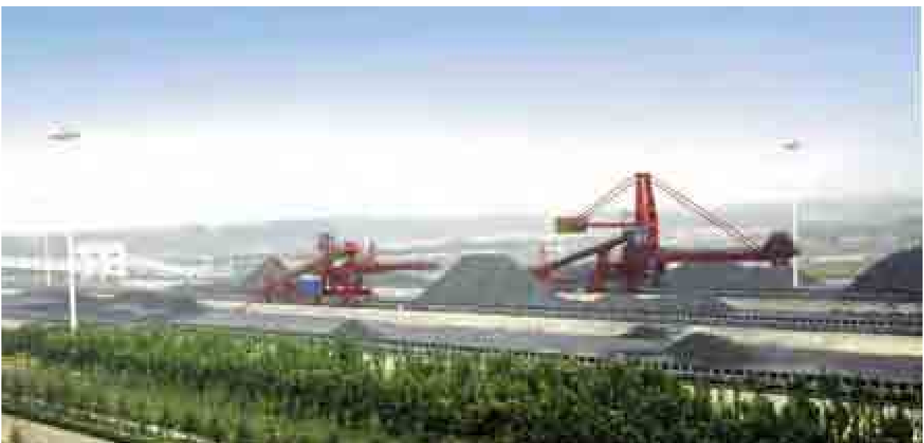
Panoramic view of the Jining Sime Darby Port (North Port) with the three iconic bucket wheel stacker and reclaimers in the background
